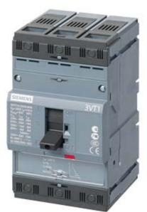
circuit breaker 3VT1 standard breaking capacity Icu=25kA, 415V AC 3-pole, motor protection trip unit TM, LI In=20A rated current IR=16...20A overload protection II=200A, short-circuit prot. without auxiliary release without auxiliary/alarm switch with front terminals
