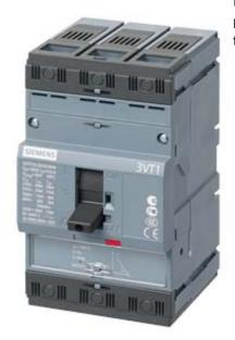
circuit breaker 3VT1 standard breaking capacity lcu=25kA, 415V AC 3-pole, line protection trip unit TM, LI In=32A rated current IR=25...32A overload protection II=160...320A, short-circuit protection without auxiliary release without auxiliary/alarm switch with front terminals
