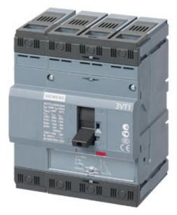
circuit breaker 3VT1 standard breaking capacity Icu=25kA, 415V AC 4-pole, line protection trip unit TM, LI In=32A rated current IR=25...32A overload protection II=160...320A, short-circuit protection N conductor unprotected without auxiliary release without auxiliary/alarm switch with front terminals
