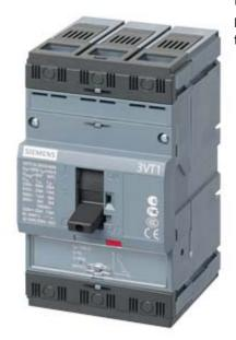
circuit breaker 3VT1 standard breaking capacity Icu=25kA, 415V AC 3-pole, line protection trip unit TM, LI In=40A rated current IR=32...40A overload protection II=200...400A, short-circuit protection without auxiliary release without auxiliary/alarm switch with front terminals
