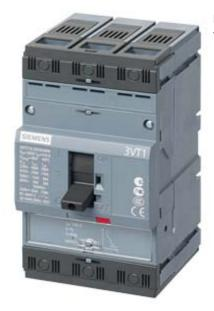
circuit breaker 3VT1 standard breaking capacity lcu=25kA, 415V AC 3-pole, line protection trip unit TM, LI In=50A rated current IR=40...50A overload protection II=250...500A, short-circuit protection without auxiliary release without auxiliary/alarm switch with front terminals
