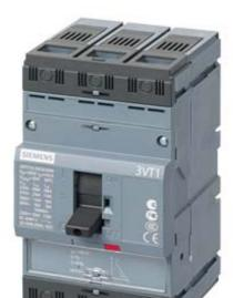
circuit breaker 3VT1 standard breaking capacity Icu=25kA, 415V AC 3-pole, motor protection trip unit TM, LI In=50A rated current IR=40...50A overload protection II=500A, short-circuit prot. without auxiliary release without auxiliary/alarm switch with front terminals
