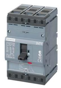
circuit breaker 3VT1 standard breaking capacity Icu=25kA, 415V AC 3-pole, line protection trip unit TM, LI In=100A rated current IR=80...100A overload prot. II=500...1000A, short-circuit protection without auxiliary release without auxiliary/alarm switch with front terminals
