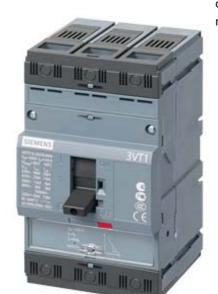
circuit breaker 3VT1 standard breaking capacity Icu=25kA, 415V AC 3-pole, line protection trip unit TM, LI In=160A rated current IR=160A overload protection II=640A, short-circuit prot. without auxiliary release without auxiliary/alarm switch with front terminals
