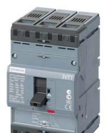
circuit breaker 3VT1 standard breaking capacity Icu=25kA, 415V AC 3-pole, starter combination trip unit TM, LIN In=160A rated current II=800...1600A, short-circuit protection without auxiliary release without auxiliary/alarm switch with front terminals
