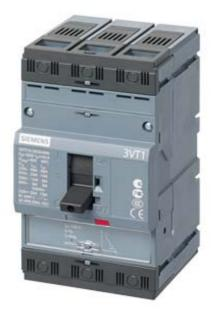
circuit breaker 3VT1 standard breaking capacity Icu=25kA, 415V AC 3-pole, line protection trip unit TM, LI In=160A rated current IR=125...160A overload prot. II=800...1600A, short-circuit protection without auxiliary release without auxiliary/alarm switch with front terminals
