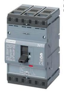
circuit breaker 3VT1 standard breaking capacity Icu=25kA, 415V AC 3-pole, line protection trip unit TM, LI In=25A rated current IR=20...25A overload protection II=250...375A, short-circuit protection without auxiliary release without auxiliary/alarm switch with front terminals
