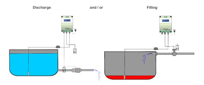
SECU Tank Relay is fulfilling the requirements of DWA-A 791-1 with clear indication of the level in the tank with high accuracy.
