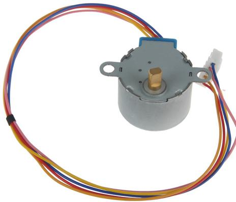
The stepper motor is an independent module that you will have to connect to the board. We need to take the stepper motor that came with the kit and connect it to our Joy-Pi.
