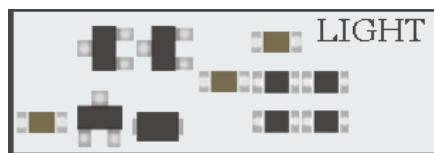
The light sensor is difficult to detect because it consists of very small parts. The sensor is to the left of the buzzer. If you cover it with your finger, the output of the light sensor should be close to zero, as no light can reach it.
