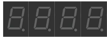
The segment LED is a very useful display when it comes to numbers and data. It can show us the time, count how many times we have done certain things. The segment display is also used in many industrial solutions, such as elevators.
