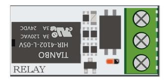
The relay is located in the middle, lower part of the board, next to the key matrix. It has 3 inputs of which we will use 2 in this example.
