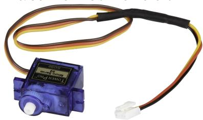
With the help of the servo motor, devices can be mechanically controlled and parts can be moved. For example, intelligent waste bins, a box with an intelligent opening and closing door and many other interesting projects can be created.
