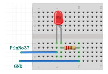
You can use this picture as a guide to create your circuit on the plug-in board. Remember that pin number 37 is on the GPIO port and GND is on the GND port of the SERVO1 interface.
