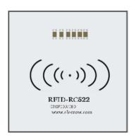
The RFID module is located directly under the Raspberry Pi and looks like a small Wifi symbol. This symbol means wireless connectivity. To use it, we need to take the chip, or card, that comes with the Joy-Pi and hold it over the Joy-Pi RFID chip area. It must be close enough for our script to be recognized. 2-4cm should be close enough. Just try it out!
