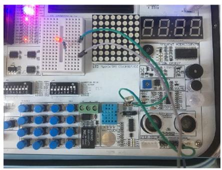
After you build the circuit ist time to write the code that will controll the LED. The plan is to send **GPIO.HIGH** to the GPIO37 Pin then wait 0.2 seconds and cut the signal with **GPIO.LOW**. This will be looped and the LED will start blinking. You can stop the programm by clicking CTRL+C.
