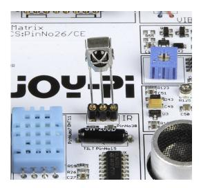
In this lesson, we will learn how to use the infrared receiver and how to receive IR codes from a remote control. The use of this method is extremely useful because we can use different define actions for different buttons. With a remote control we can switch on different LEDs or control the servo motor each time the button is pressed.
