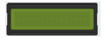
The LCD screen takes up a large part of the Joy-Pi board - it is located at the top center of the Joy-Pi, to the right of the GPIO LED display. As soon as the demo script and the examples are executed, the display turns on. Thanks to the integrated backlight you can read data on the display even in complete darkness.
