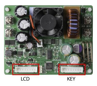
First connect the display module with the enclosed cables to the corresponding LCD and key interface. In the next step, you can connect the inputs and outputs to the device via the screw terminals.
