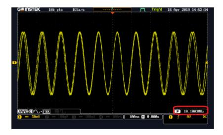
B. Set the center frequency of the Spectrum Analyzer by this frequency; set the start and stop frequencies to clearly observe the changing waveform of the FSK in the frequency domain.
