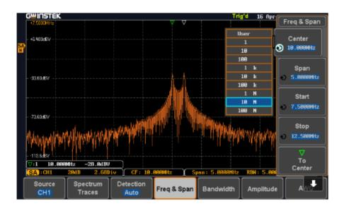
C. Use the search function to find Max.peak to clearly display the measurement data.
