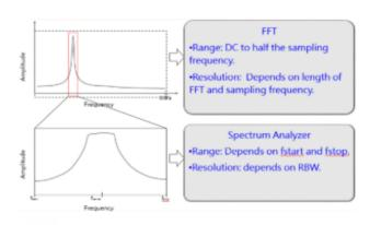
For users who have not used a spectrum analyzer before, the parameters on the spectrum analyzer could be unfamiliar.
