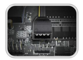
Synchronizing all RGB lighting devices on your system with the +12V RGB header. (+5V RGB header is not supported by this model)
