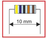
**Bend the resistor wires so they slide easily between the lands**
