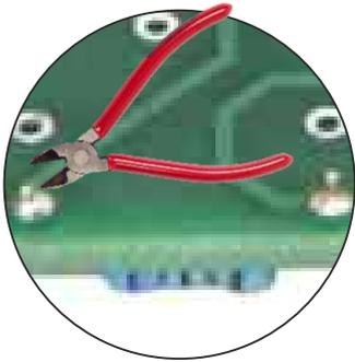
After soldering, use wire cutters to trim the excess wires at the back to approx. 2 mm.
