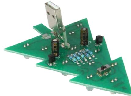
**H** After choosing the correct position you can solder the USB connector in place. First slightly solder in one area, adjust the USB connector (if crooked), then solder on the other 3 areas. Once all 4 points have been soldered, the USB will then be firmly attached.
