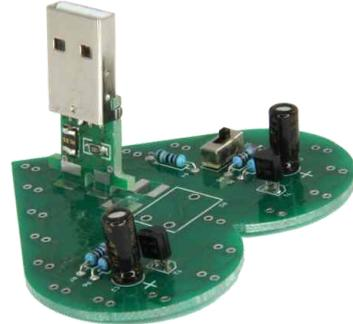
**G** After choosing the correct position you can solder the USB connector in place. First slightly solder in one area, adjust the USB connector (if crooked), then solder on the other 3 areas. Once all 4 points have been soldered, the USB will then be firmly attached.
