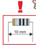
**Bend the resistor wires so they slide easily between the lands!**
