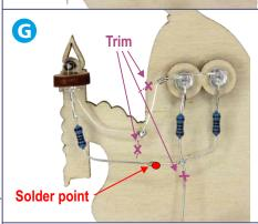
Trim the excess wire for the positive contacts and solder on the last resistor as shown.
