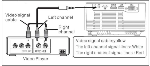
**Audio output:** Audio signal from the output port of the device, if you want to high power play music input end connected to external power amplifier.
