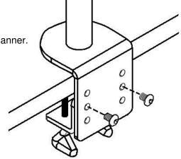
**40695:** Single short bracket – Max 10kgs each monitor **40696:** Single long bracket – Max 10kgs each monitor **40697:** Double long bracket – Max 6kgs each monitor
