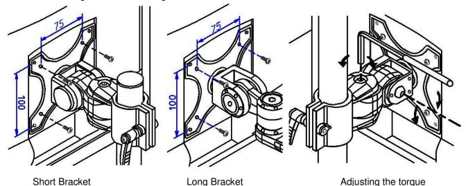
Both the long and short brackets attach to your monitor in the same way using the screws provided
