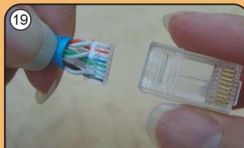
To arrange the plug body
