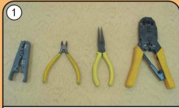
Tools : Stripper, Cutter , Pliers, and Crimping Tool
