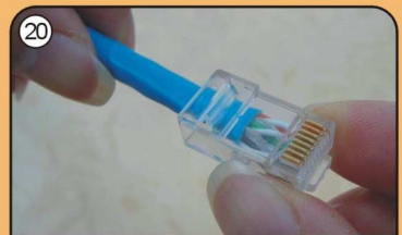
To put the plug body into the insert/cable
