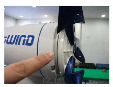
6. Attach the nose cone by pressing it against the hub
