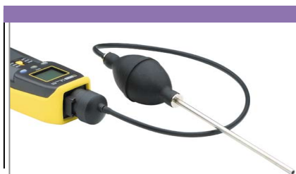
Gas extraction kit with pump and connector
