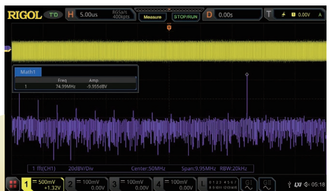
With the near-field probe, you can easily observe the spectrum peak in the frequency domain when the probe approaches to the radiation leakage point.
