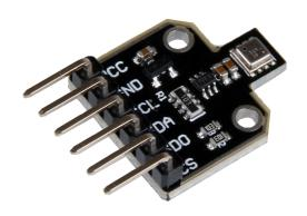
The BME680 from Bosch Sensortec is the new, compact ambient sensor with integrated sensor technology for light humidity, pressure, temperature and air quality.
