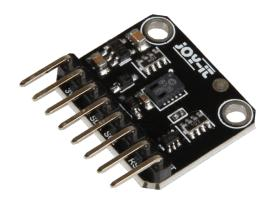
The CCS811 is a gas sensor that monitors the air quality and can measure a large number of volatile organic compounds (VOCs).
