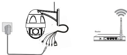
Once you've added your camera successfully using the wired connection method above, tap your live camera feed from the **My Cameras** screen > tap the gear in the upper-right > tap **Network** > tap the WiFi network you wish to connect to and enter your WiFi password.
