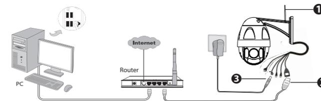
**Note:** We highly recommend that you first begin the setup process by connecting your camera to your Internet router with an Ethernet cable. After setup is successful, you'll be able to unplug the cable and login to your wireless network for WiFi operability.
