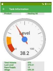
The ECO-MAT allows to check the level in liquid tanks and monitor them.
