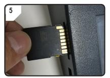
Insert the SD card with the label facing downwards.
