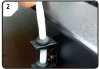
· Insert the filament tube into the tube holder.
