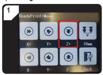
In the < ReadyPrint > menu, select < Move > and then press < Z+ > twice to increase the distance between the nozzle and the print bed.
