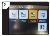
Select < 115200 > to control the 3D printer via the control panel.
