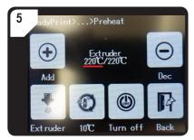
Wait until the actual temperature (in this case 220 °C) has reached the target temperature.
