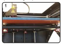
• Tighten the 3 levelling screws under the print bed as far as they will go.
