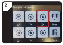
• In the < ReadyPrint > menu, select < Move > and then press < Z+ > twice to increase the distance between the nozzle and the print bed.
