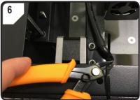
• Cut through the cable tie on both sides using the wide cutter.
