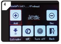
Press < Add > several times until the target temperature of 220 °C is reached.
