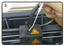
Insert the filament into the tube until approximately 5 cm is visible at the end of the extruder.
