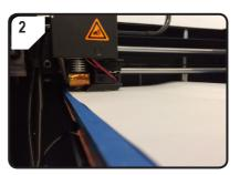
Place an A4 sheet of paper between the nozzle and the print bed to use as a measurement quide.
