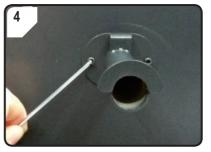
Use two screws and the 2.5 mm hex key to attach the filament spool holder to the back of the 3D printer.
