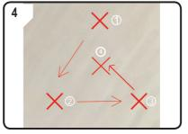
Repeat step 3 for the second, third, and fourth point (calibration sequence and motion direction of the nozzle are shown above).
