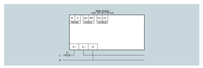
\* The fuse in the voltage measuring input is only used for cable protection.
