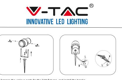
1.Arrange the various parts for the light fixtures, and install the bracke 2.Distinguish positive, negative electrode and earth wire between the power cord and the luminaire.
