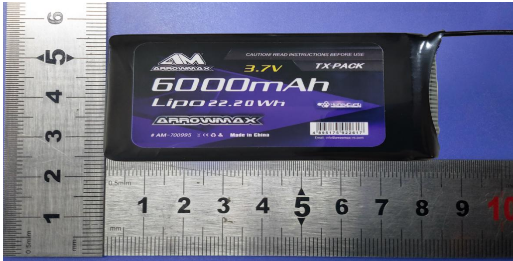
Battery (AM-700995 3.7V 6000mAh 22.2Wh)
