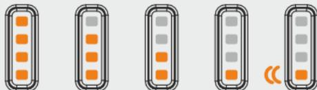
The orange LEDs show current battery level: >75%, >50%, >25% or >3%.
