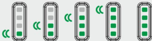
Always you can see an actual charge level. Green light blinking shows which charge stage is going: >0%, >25%, >50% or >75%.
