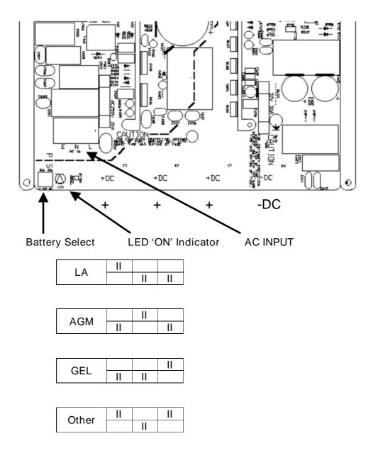
FIGURE 1 INPUT/OUTPUT CONNECTIONS
