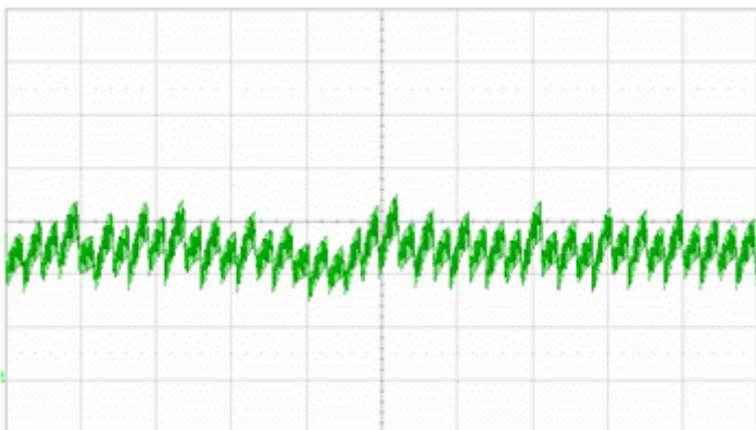
Running current at 48,0 V; 7.000 1/min; I=500mA/Div, t=2ms/Div
