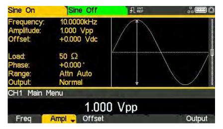
The amplitude can be set in terms of peak-to-peak Volts (Vpp) from the **Ampl** soft key, to set high and low levels see 'High level and low level'. The level can be set assuming that the output is either open-circuit or terminated.
