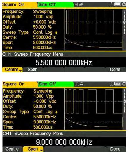
With centre/span mode selected the Edit Box shows the parameter, the Parameters Box shows **Centre** and **Span** in place of **Start** and **Stop** and the Graph Box changes to show the parameter which is being edited.
