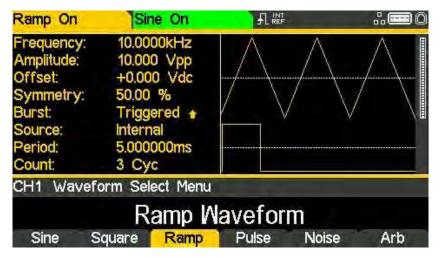
In the Output menu, press the **Phase** soft-key to change the start phase of the waveform. The phase parameter will appear in the Edit Box.
