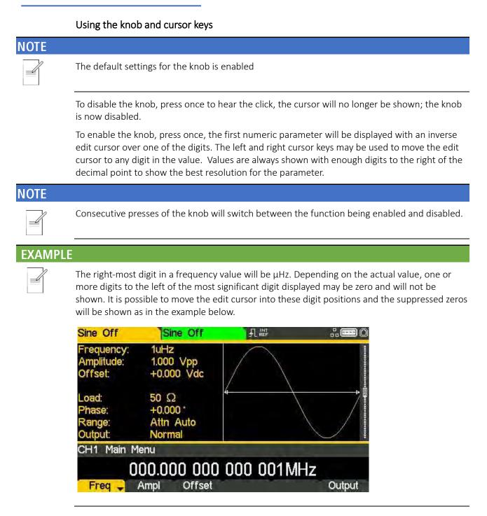
With the edit cursor positioned at the required digit the knob may be rotated left or right to decrement or increment the digit. As the value passes between 9 and 0 the digits to the left will also change. In this way it is possible to set any legal value for the parameter.
