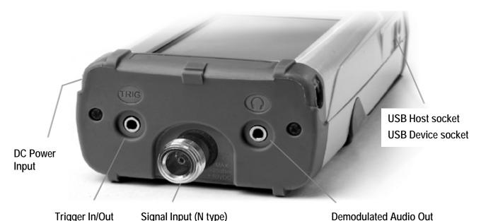
**DC Power Input** 1.3mm power socket mounted on the right hand side of the instrument.
