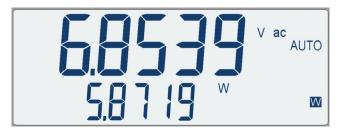
The VA function makes use of the dual measurement capability and displays the product of voltage and current.
