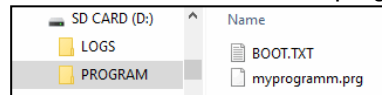
Fig. 68: microSD memory card drive with PROGRAM folder contains BOOT.TXT and compiled test.prg program
