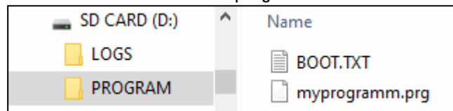
Fig. 66: microSD memory card drive with PROGRAM folder contains BOOT.TXT and compiled test.prg program
