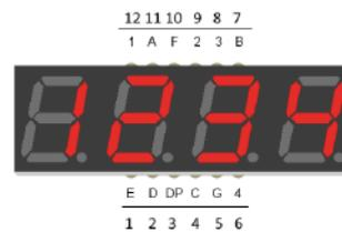
The connections on the seven-segment display.
