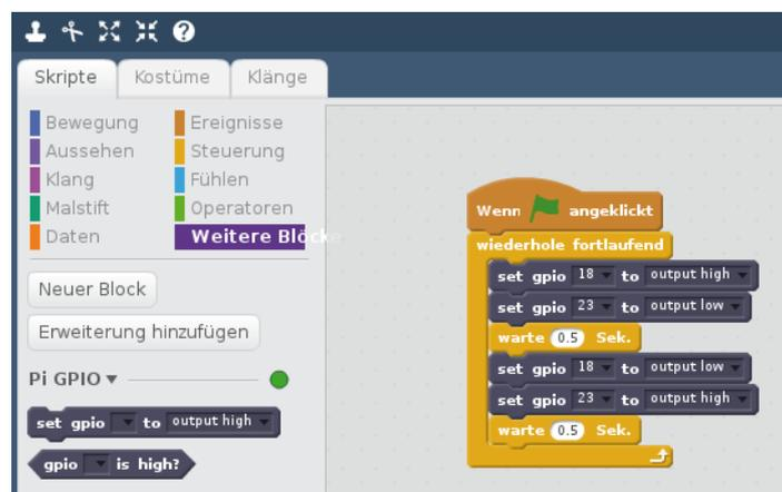
This Scratch program 02Led02 flashes two LEDs alternately.
