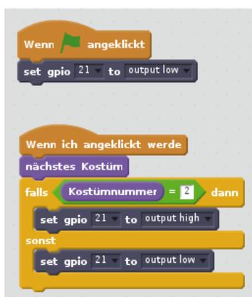
Scratch blocks for segment A of the seven-segment display
