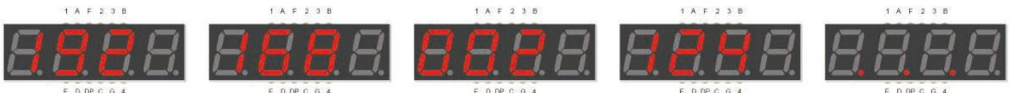
Display sequence of an IP address on the seven-segment display.
