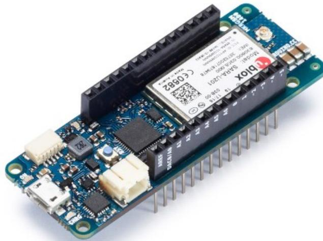
**Arduino MKR GSM 1400** has been designed to offer a practical and cost effective solution for makers seeking to add global GSM connectivity to their projects with minimal previous experience in networking. It is based on the Atmel [SAMD21](#) and a [SARA-U201](#) GSM module.
