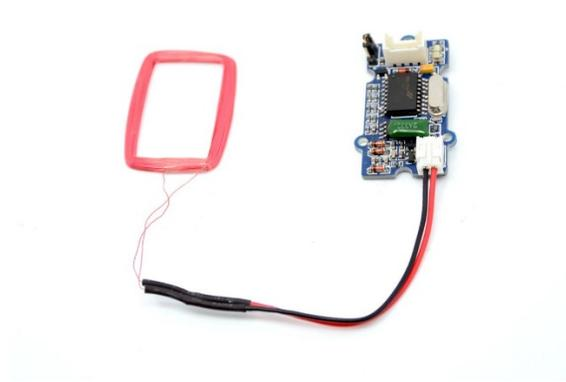
This Grove-125KHz RFID Reader is a module used to read uem4100 RFID card information with two output formats: Uart and Wiegand. It has a sensitivity with maximum 7cm sensing distance. There is also [the electronic brick version](#) of this module. It can help you with project like internet of thing and access control system.
