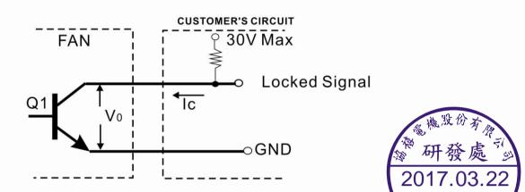
\*Transistor Q1 at "ON" position Collector current.....I<sub>c</sub>=10mA Max Saturation Voltage.....V<sub>oL</sub>=1.0V Max (Between Collector and Emitter at I<sub>c</sub>=10mA) \*Transistor Q1 at "OFF" position Release Voltage.....V<sub>OH</sub>=30V Max
