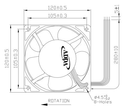
LEAD WIRES: UL 1061, AWG24; L = 280±10 mm
