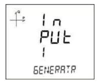
3. Pulse Input: When this option is selected, the device can count the pulses that occur on the input. It can display the pulse count on monitoring screens under "Pulse Cntr C-1" section.
