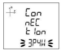
1. By using UP/DOWN buttons, select your network connection type as 3P4W, 3P3W, ARON, 3P4W Balanced or 3P3W Balanced.
