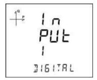
2. Generator Input: When this option is selected, the device records the energy to the generator register depending on the input state.
