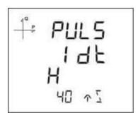
For devices with pulse counting feature, the minimum time necessary for the pulse counting can be selected from following options:
