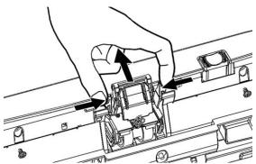
3. Install the new pad module by inserting the tabs on the module onto their slots on the scanner.
