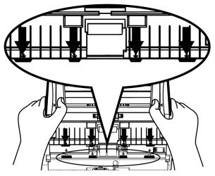
3. Close the panel unit by pushing it back down until it snaps back into place.
