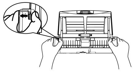
3. Remove the feed roller by pinching the feed roller and pull it out.
