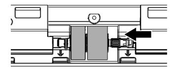
4. Install the new feed roller by aligning and inserting the feed roller onto the roller pitman on the scanner.
