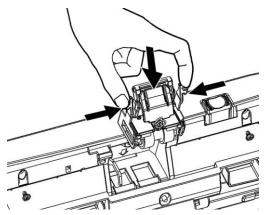
4. Close the panel unit by pushing it back down until it snaps back into place.
