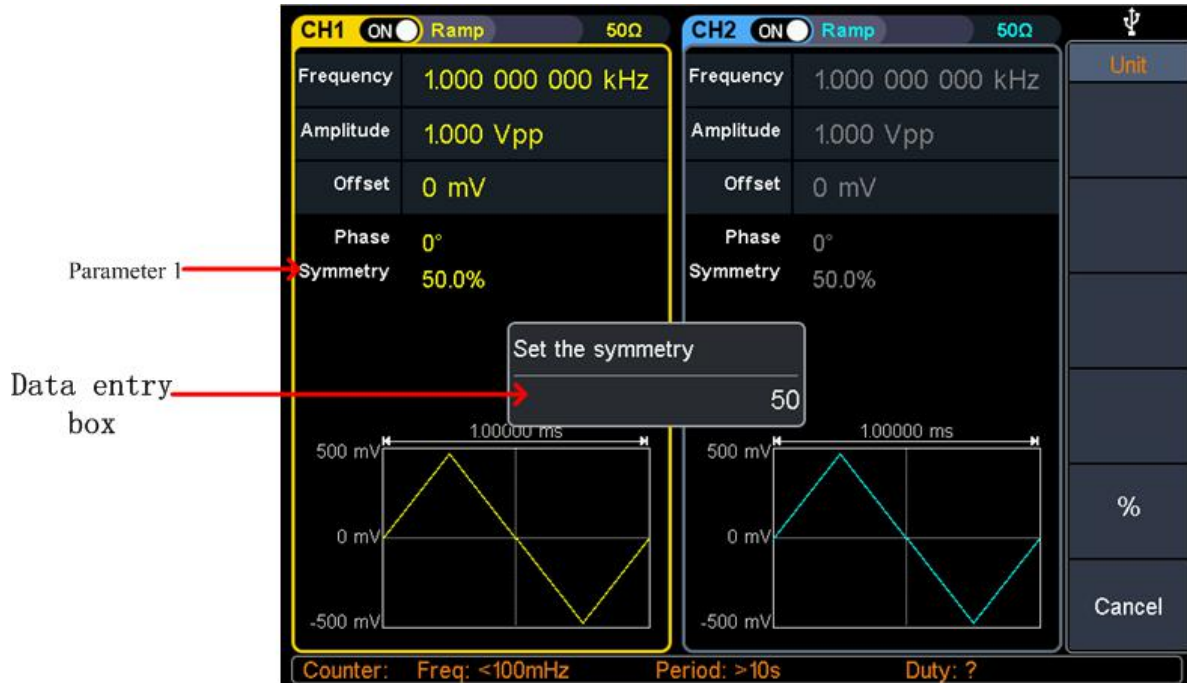
Figure 4- 5: Set the symmetry of ramp wave
