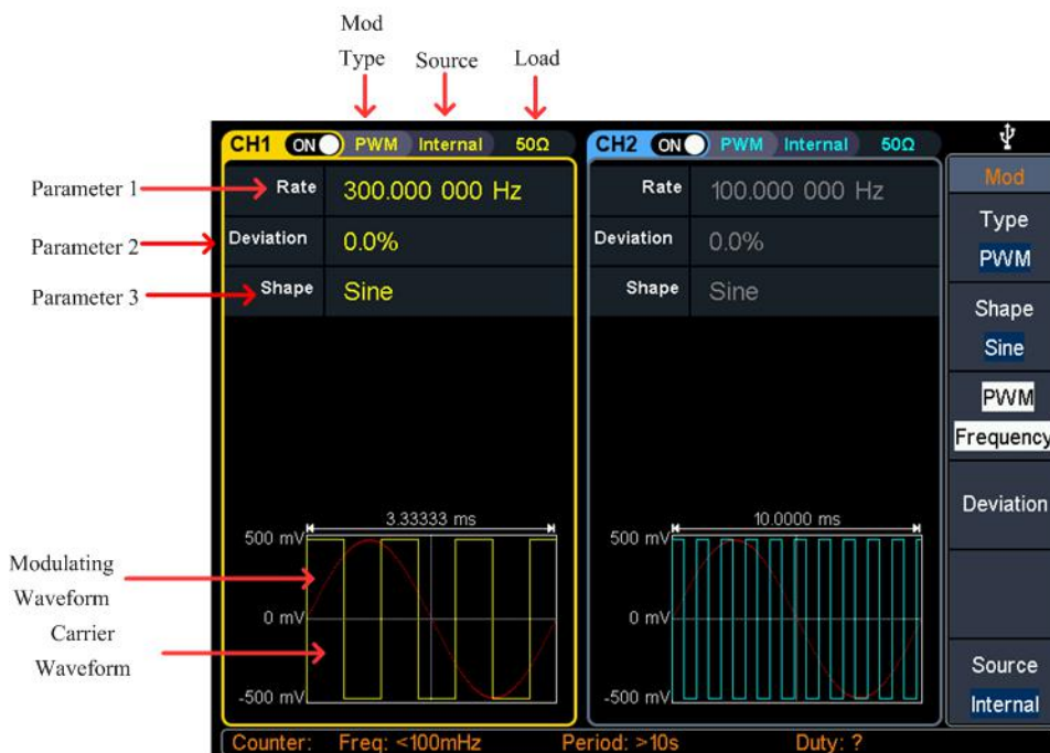
Figure 4- 14 Pulse width modulation user interface
